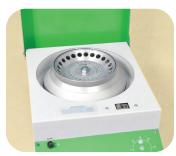
Immediately remove a portion of the top layer of extract and centrifuge it for 30 seconds at 2000 x g (NOT RPM).
