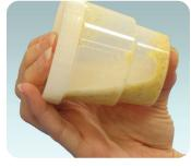
Immediately shake vigorously to dissolve pouch, then shake an additional 1 minute on mechanical shaker (or by hand for 2 minutes).
