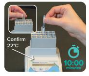
Place tube in Incubator and acclimate for 2 minutes\* before adding TotalTarget Enogen Strip; wait **10 minutes** for results.
